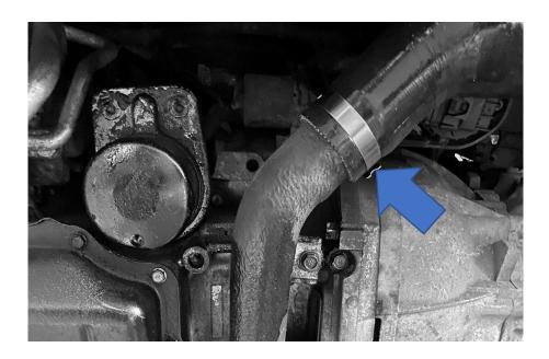
2. Locate the boost pipe coming from the turbo and release the hose clip. You may need to remove a cap over the end of the clip using a pair of pliers or grips to pull it off.
