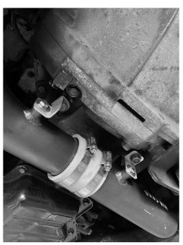
7. Finally, once happy with the positioning of the pipework and silicone hoses proceed to tighten the brackets followed by all of the jubilee clips.
