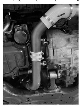
6. Install the brackets onto the car using the 12mm volts removed in Step 3 and then attach the brackets using the supplied M6 bolts and washers, as shown.
