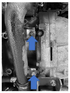
4. Remove the existing Pro Hoses silicone hose and then reinstall it directly onto the turbo with the longer of the two hard pipes supplied, as shown. Do not tighten the jubilee clips yet.
