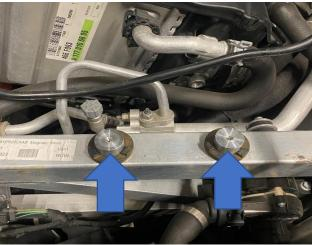
8. Fit the air box bases in place and install using one M6x25mm Button Head bolt with washer (blue arrows) and two M6x16mm Button Head bolts with washers (orange arrows) each side.
