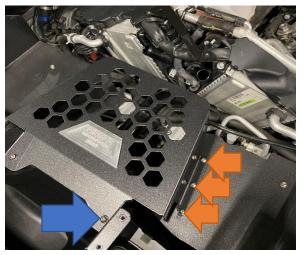
10. Using an M6 Button Head bolt with washer, fit the supplied bracket extension in place where the right-hand 13mm stud was removed in Step 1 but leave it loose to allow movement.
