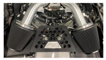
16. Finally, fit the air box lids using the 10x M5mm Button Head bolts supplied and check everything is tight.
