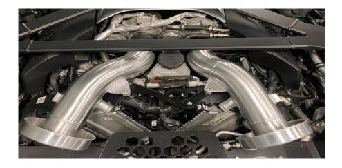
12. Fit the replacement Pro Hoses recirculation hoses using the supplied 35mm jubilee clips.
