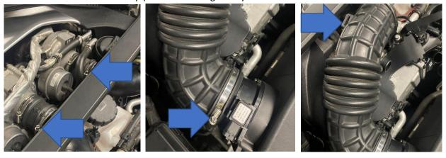
5. Now release the two air boxes by removing the two 8mm bolts on top and then pulling it firmly but carefully up to release the push fits underneath. Also unclip the small hose fitted to the back of the right-hand air box.
