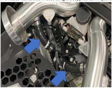
13. Remove the MAP sensors from original air boxes by twisting and pulling them carefully.
