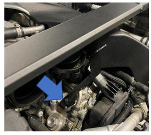
7. Insert the four AIRTEC Motorsport alloy push-fittings by pushing into original air box bushings, as pictured.
