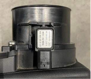
14. Insert the MAP sensors into the new pipes in reverse of Step 13 and then clip the wiring back into place.
