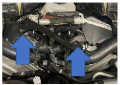
2. Now remove both the left- and right-hand recirculation hoses at the front of the engine. Use hose clamp pliers or large pliers to loosen all four of the clamps and then remove the hoses from the engine bay.
