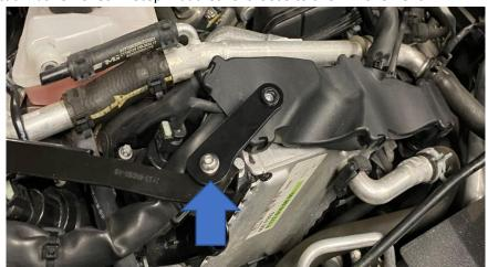
11. Guide each of the new intake pipes into place by fitting them into the turbo inlets first and then rotating them to line up with the mountings. Once happy with the fitment, reuse the original jubilee clips and fit the supplied M6 Socket Head bolts. Do this for both sides, then fully tighten the extension bracket bolt.
