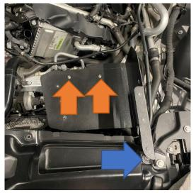
9. Place the centre section so that it overlaps both base shields equally and line the eight holes up in the centre. Use two M6x25mm Button Head bolts with washers (blue arrows) and six M6x16mm Button Head bolts with washers (orange arrows) to secure it in place.
