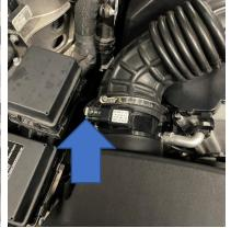
4. Loosen the four jubilee clips that connect induction pipes at both ends, then release the hoses from the location tabs and remove the pipes from the engine bay.
