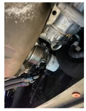
15. Finally, the air feed hose can now be fitted to the oil cooler scoop and feed using the provided jubilee clips. You will then need to fill an extra half litre of oil to the engine before starting. Once up to temperature, check the oil level again.
