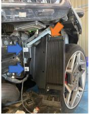
8. Install the second bracket with the AIRTEC logo onto the oil cooler as shown and secure using the M6x16mm Button Heads bolts, Nyloc nuts and washers. Four are fitted to the end brackets (highlighted in blue) and another two (highlighted in orange) sandwich the two brackets together. Make sure only the one tab (highlighted in blue) is without a bolt, as this will be used to secure another bracket.
