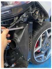
11. Remove the undertray to gain access to the torque mount and oil filter by undoing the eight fixings. Then you will need to remove the bolt from the front of the torque mount using a 16mm socket to allow extra access to the oil filter at the front.
