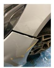
3. Release the six plastic trim clips from underneath the front bumper, then unplug the wiring harness for the fog lights and lift the front bumper off and away from the car with the help of another person.
