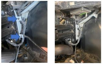
5. Remove the left-hand side arch liner to give more access by undoing two 10mm bolts in the undertray and the seven plastic trim clips inside the liner. There is also one T20 Torx bolt securing the side skirt cover to the arch liner.
