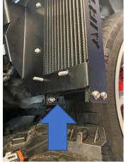
9. Now install the support bracket in place by using two M6x16mm Hex Head bolts with washers and Nyloc nuts.
