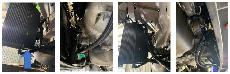
14. Now reinstall the oil filter and check that the oil lines, fittings and the filter have all been fully tightened and secured in place correctly to avoid any leaks. The torque mount bolt can now be reinstalled and the undertray refitted in reverse of Step 11.
