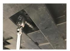
8 Release the six plastic trim clips from underneath the front bumper then unplug the wiring harness and carefully remove the front bumper.
