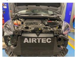
12 Finally, check fitment is secure and then refit the front bumper in reverse of Steps 5 to 7.
