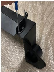
3. The final divider can now be installed on top of the air feed scoop. This will go in the centre of the air guide. Once in place, secure using the M5x12mm Button Head bolts with washers and Nyloc nuts.
