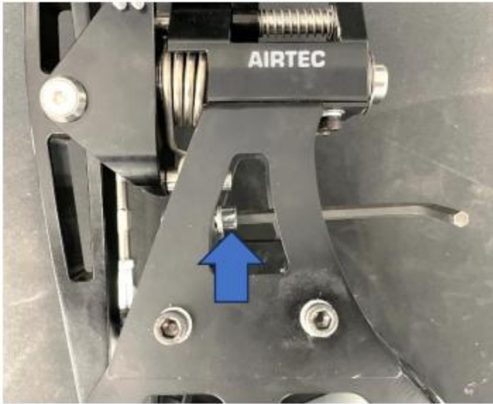
Side view of bolt to adjust with Allen Key in place.
