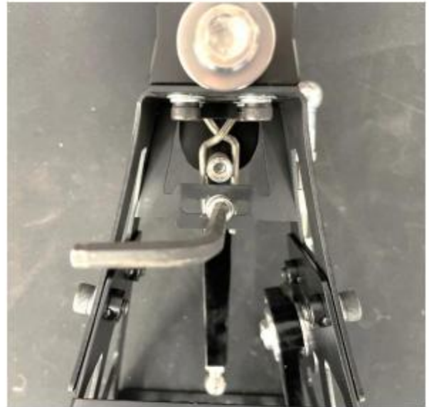
Rear view of bolt to adjust with Allen Key in place.
