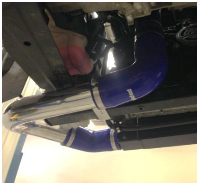
Right-hand side uses larger diameter pipework
