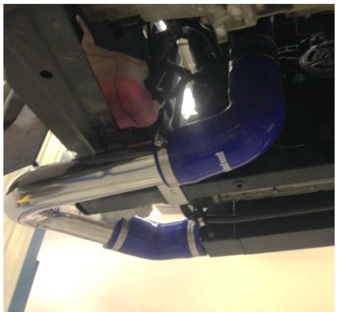
Right-hand side uses larger diameter pipework
