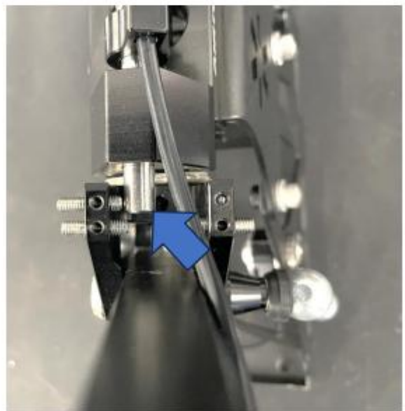
When you lift the lever's reverse collar the centre bar should move back to allow reverse to engage.
