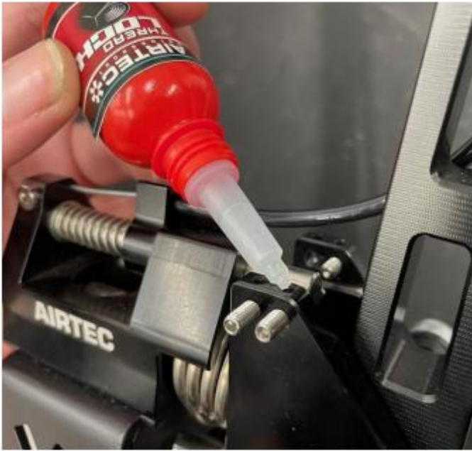
Apply a good amount of Lock Thread to each of the holes.
