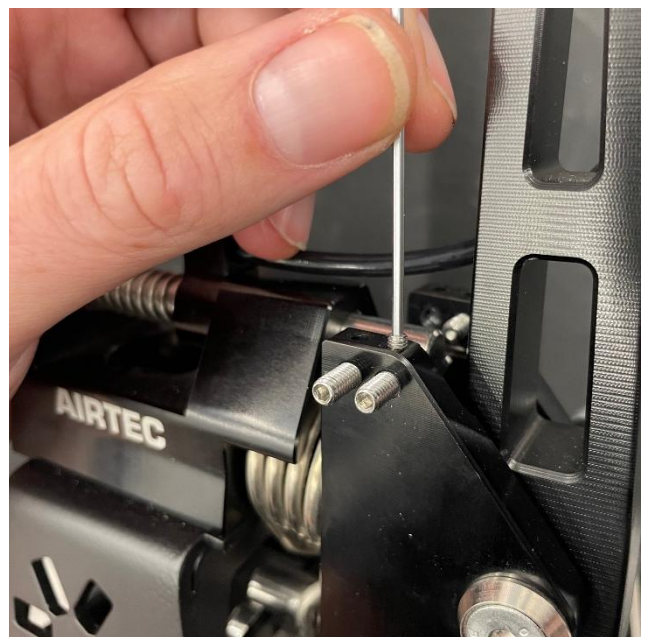
Use the supplied Allen Key to screw in the top grub screws.
