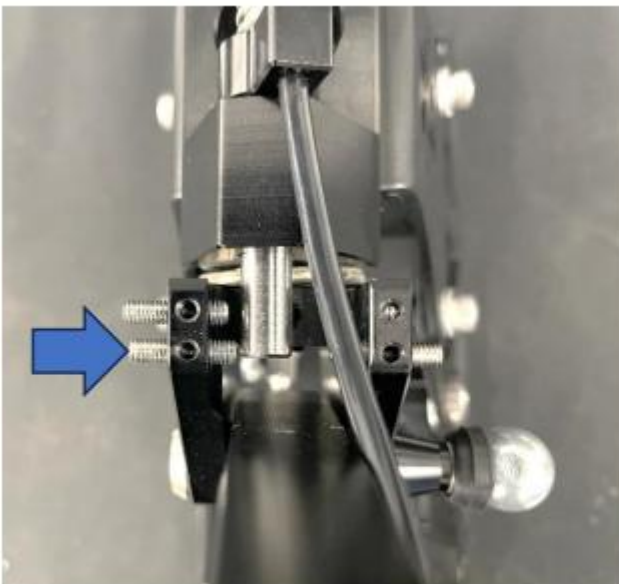
Select sixth, insert a grub screw in the lower left hole until it reaches the centre bar and unwind half a turn.
