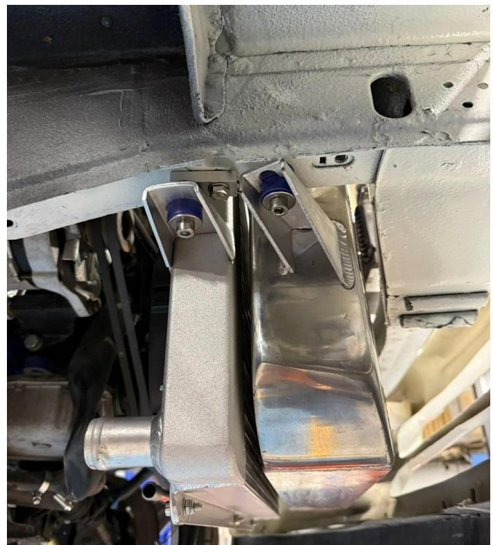
You can then mount the radiator to the rear mounting holes, as shown. Please note: The optional mounting bush kit is shown here.
