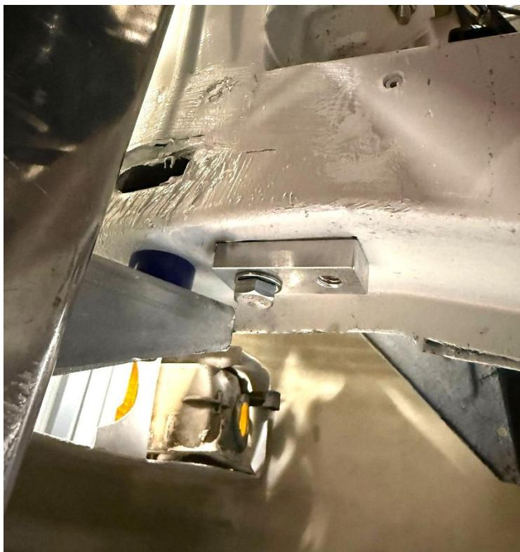
Place the intercooler in front mounting holes and then use the other hole to mount the bracket.
