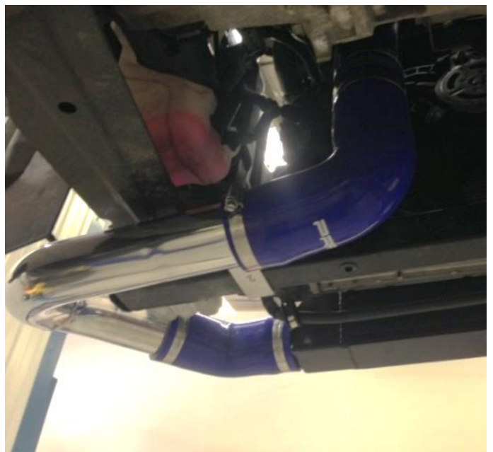
Right-hand side uses larger diameter pipework
