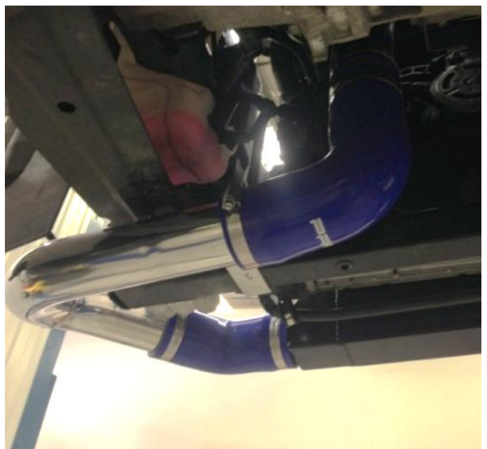
Right-hand side uses larger diameter pipework
