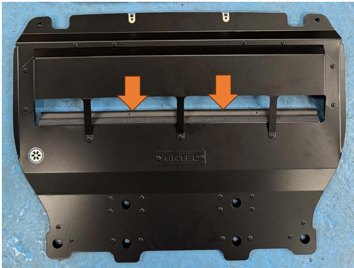
3. Finally, mount new aluminium under tray using all the original under tray fixings.
