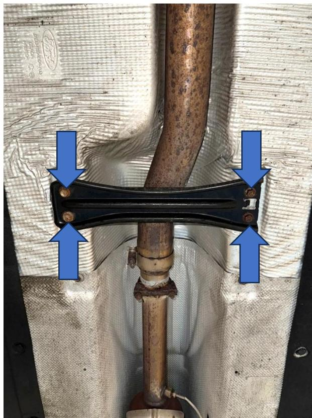
2. Now install the new AIRTEC Motorsport brace in the same location. If you have an aftermarket/larger exhaust system, you may need to the spacers supplied in the kit to allow clearance.
