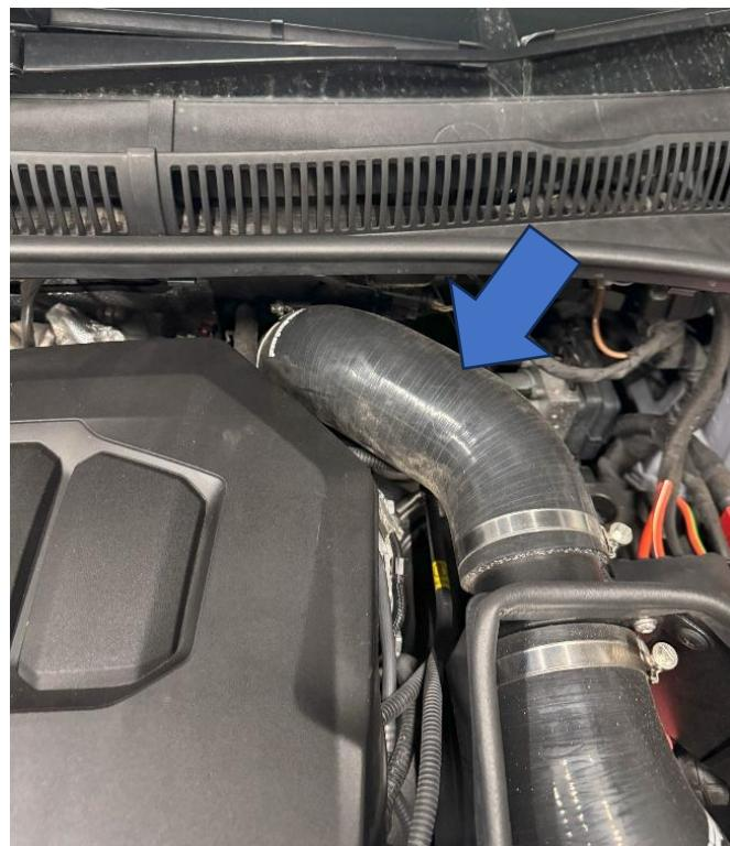
2. Remove the hose attached to the original turbo muffler by releasing the two jubilee clips.
