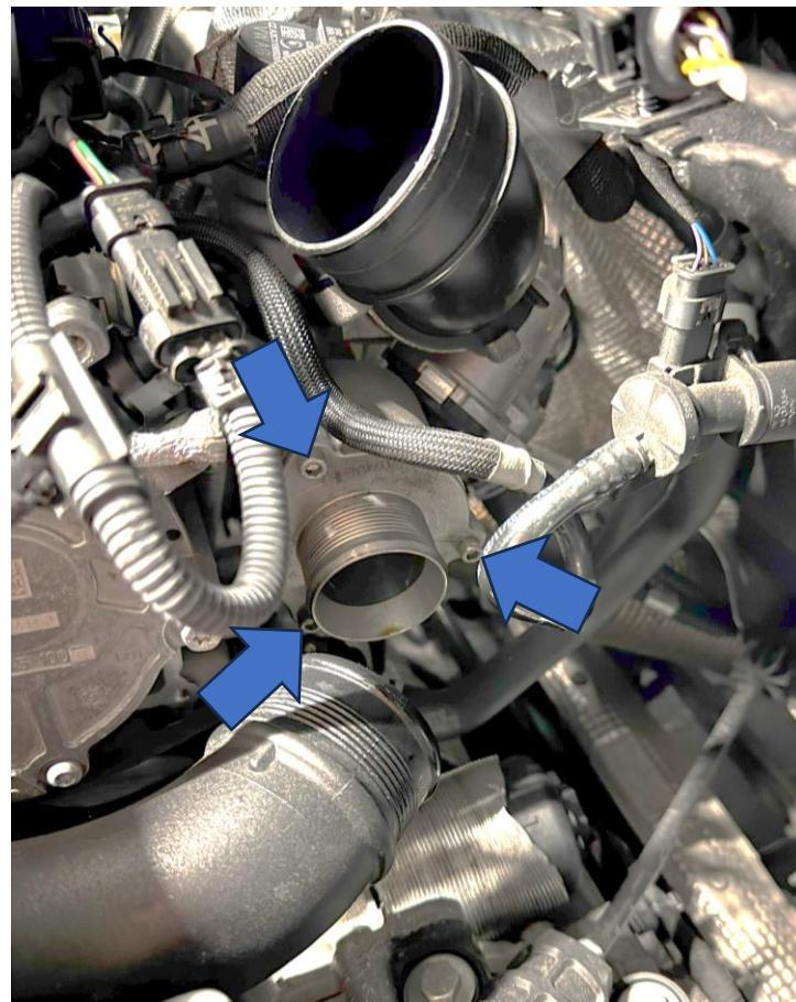
4. Before installing the new AIRTEC Motorsport muffler delete, check that the mating face is fully clean. Then offer it up and rotate until all three holes line up. You can then secure reusing the original bolts.
