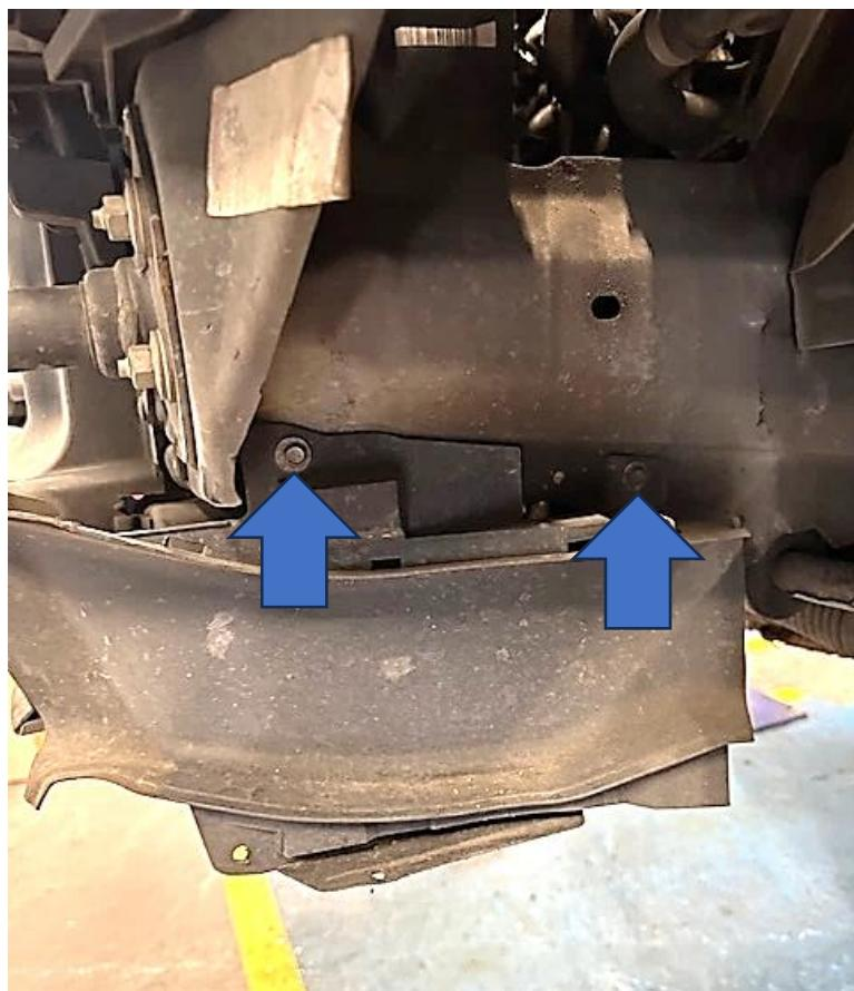
6. Remove the four cross-head push fittings and pull the radiator air guide forward to release it.
