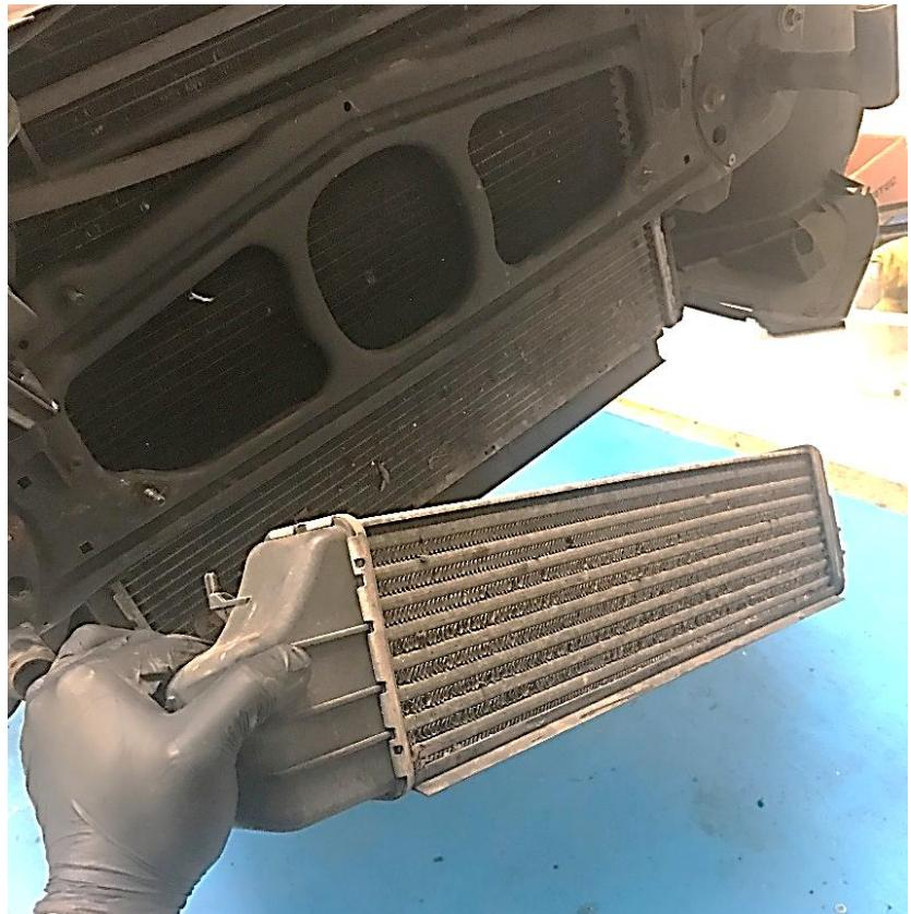
9. The original boost hoses will need removing so that the new silicone hoses can be installed. To access the cold side hose, you need to remove the air box feed by undoing the two fittings on the slam panel and then pulling the hose out before pushing it back and lifting it out.
