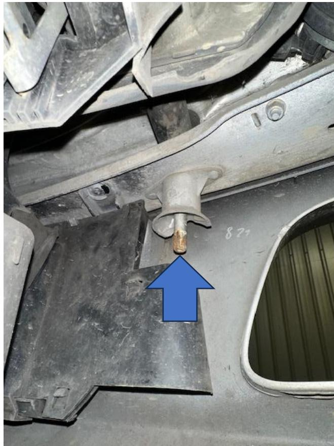
4. Now carefully unclip the edges of the bumper and pull it forwards. You will need a second person to help you unclip the horns and fog lights before you can remove it from the car.
