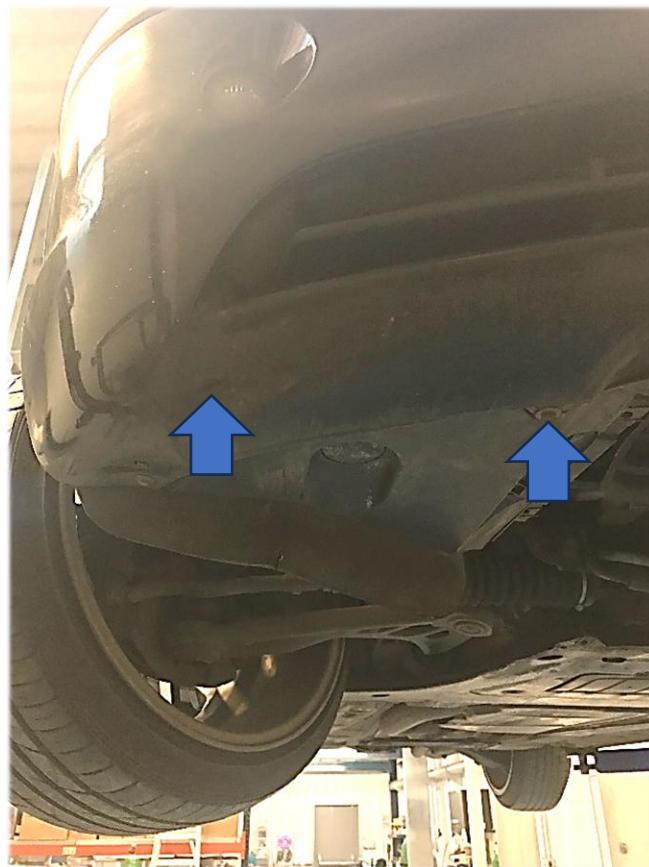
3. The final fixings to remove the bumper are two E12 Torx bolts located on the inside of the bumper. These can be accessed from underneath using a long extension bar.
