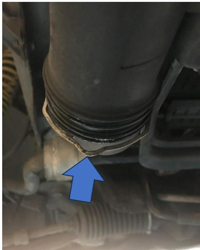
8. Underneath the intercooler there are two T20 Torx bolts securing it to the bottom of the radiator. Remove these and the intercooler will release from the car.
