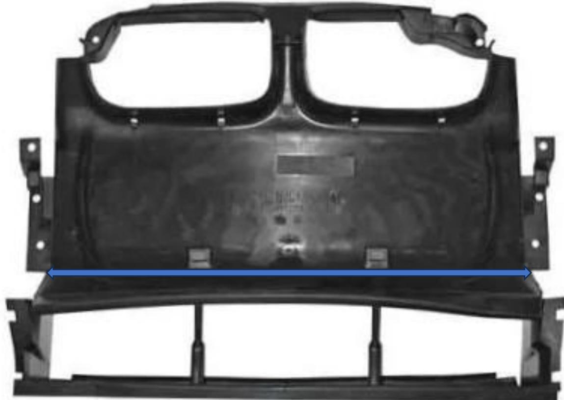
17. Depending on the model of car the intercooler is being fitted to, you **may** need to trim the inside of the bumper where it meets the intercooler, as shown. Please check before attempting refitting.
