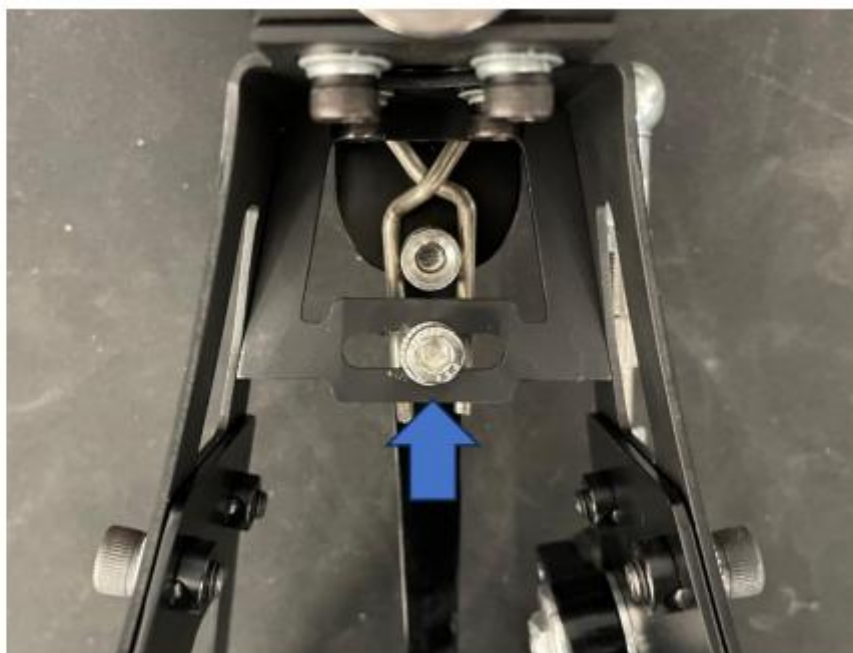
There is adjustment in the bracket to move the bolt left and right.
