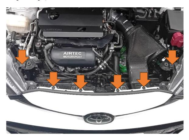
2. Fit the panel in place and secure using the original fittings removed in Step 1.
