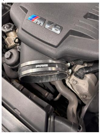
6. Now place the carbon fibre intake pipe in place by pushing it up to the lip and proceed to tighten the second jubilee clip. You can then reattach the vacuum hose removed in Step 2 by clipping it back into position.
