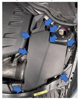
2. Undo the jubilee clip attaching the original intake pipe to the plenum (blue arrow) and release the vacuum hose from the take-off by squeezing the tabs together (orange arrow).
