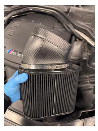
8. Place the second supplied silicone hose onto the carbon fibre intake, followed by the elbow. Be careful to ensure you line up the groove in the elbow with the air box base as shown and then tighten the jubilee clips.
