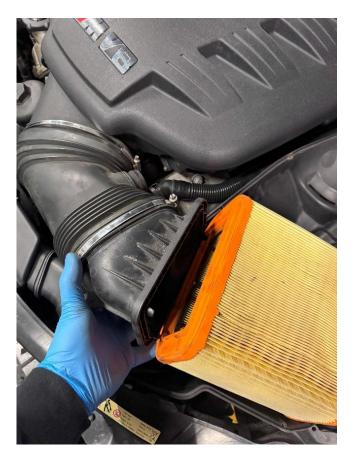
4. To make installation easier, now remove the front air feed hose by pulling it loose.
