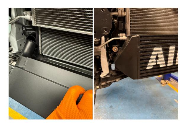
18. To refit the radiator air guides you will need to trim them using a suitable cutting tool, such as a hacksaw or Dremel. They can then be reinstalled into the vehicle and secured with the clips on the radiator.
