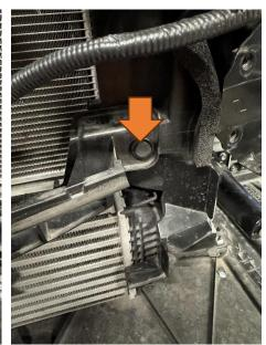
10. Now the plastic air guide on each side can be removed by lifting it up at the bottom to unhook it from the intercooler, followed by unclipping it from the radiator.
