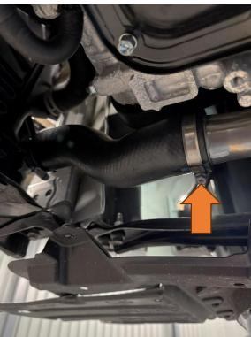
14. Remove the three 10mm bolts from the intercooler and then tilt it forwards to remove from the car.
