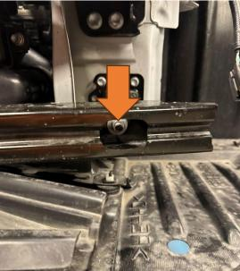
8. The crash bar can now be removed by unclipping the two wiring harness connectors using a trim removal tool, undoing the 10mm nut attaching the ambient temperature sensor bracket to the crash bar followed by the four 14mm bolts each side securing the crash bar to the car.
