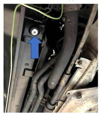
9. Then remove the power-steering lines from the clips attached to the radiator fan shroud.
