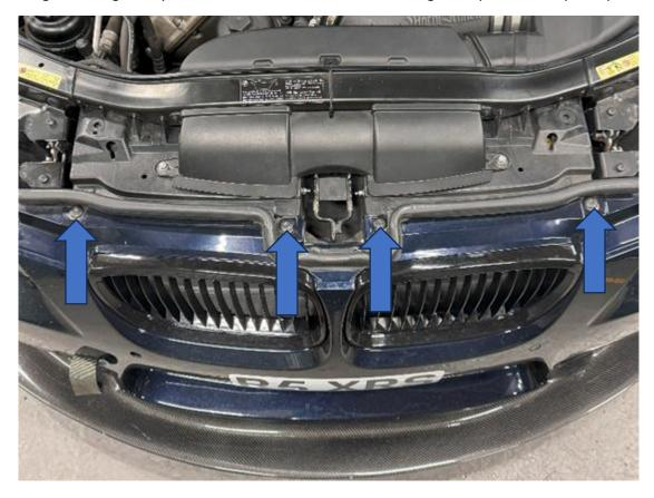
5. With the help of a second person, pull the edge of the bumper away until it releases. If your car is fitted with front parking sensors, then unclip the connectors before removing the bumper.
