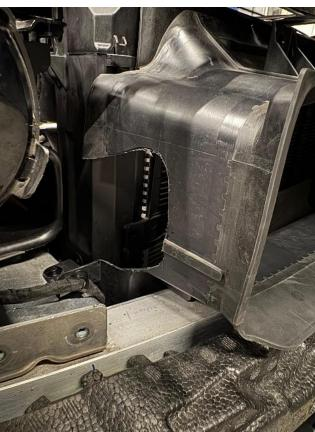
13. Now insert the scoops into the original air feed and the then mark the locations of their mounting holes on the grille frame with a scribe or fine pen, as shown.
