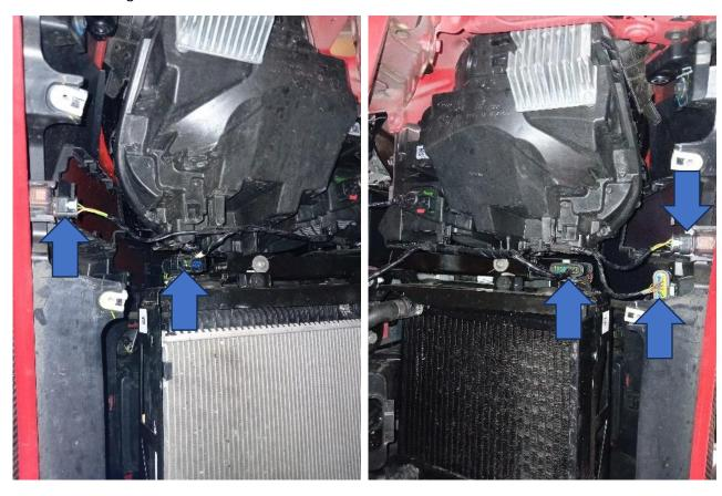
4. Working under the car, remove the rubber bumper trim by undoing the 11 self-tapper screws. There are then four plastic hook clips that slot under the front section of the bumper, so pull the bumper trim towards the back of the car to release it.
