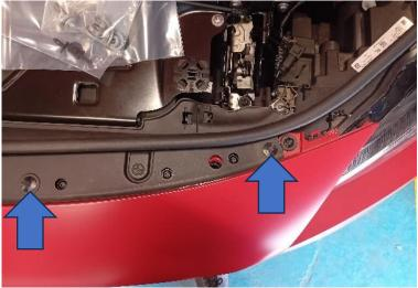
8. Remove the 10 T30 Torx screws securing the top of the bumper and then carefully lift it away from the car.
