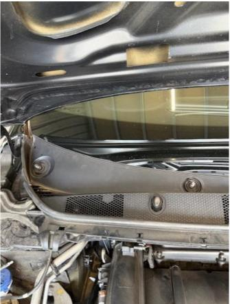
3. Now use a trim removal tool to unclip the wiring loom.
