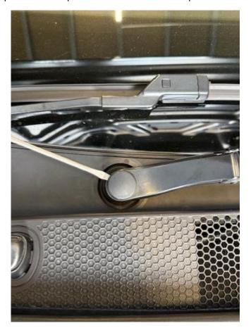
2. Unclip the front of the scuttle panel and disconnect the washer jet hose. Then carefully unclip the panel from the windscreen and lift it away.
