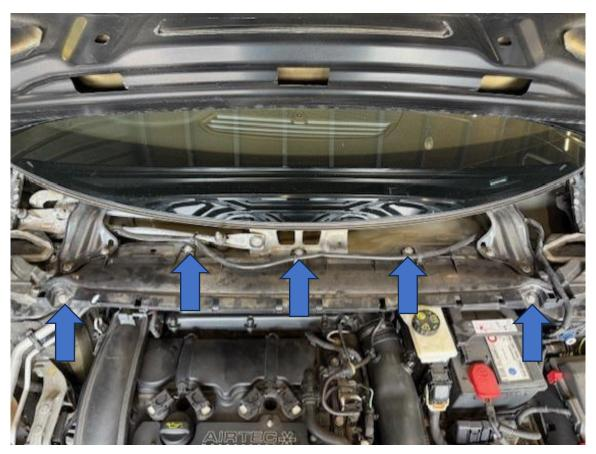
5. Carefully undo the brake reservoir using a T30 Torx and place it over the battery.
