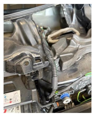
7. Next, unplug the MAF sensor and unclip the vacuum line on the air box lid.
