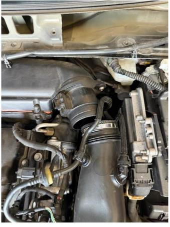
9. Fit the induction hard pipe supplied in the kit into the original intake hose, as shown. Then attach the silicone hose provided with jubilee clips, but do not fully tighten yet to allow adjustment.
