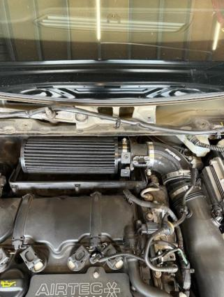
13. Connect the vacuum line fitting removed in Step 7 to the top of the new AIRTEC Motorsport air filter.
