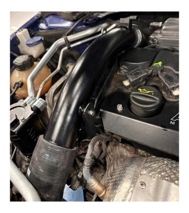
14. Remove the MAP sensor from the original pipe using an 8mm socket and then install it into your new AIRTEC Motorsport pipe using the supplied M5x12mm Socket Head bolt.
