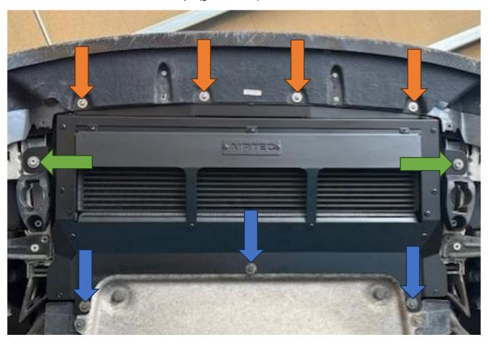
5. Finally, reinstall the left and right trim pieces removed in Step 1. But use the remaining two M5x16mm Button Head bolts with washers (blue arrows) to replace the fixings used originally.
