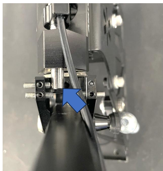
When you lift the lever's reverse collar the centre bar should move back to allow reverse to engage.
