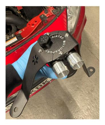
4. Install the catch can assembly onto the car and then reinstall the nut and bolt removed in Step 2.
