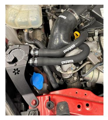
**Please note:** Check the dipstick on the catch can periodically and empty as necessary by unscrewing the base of the catch can anti-clockwise.
