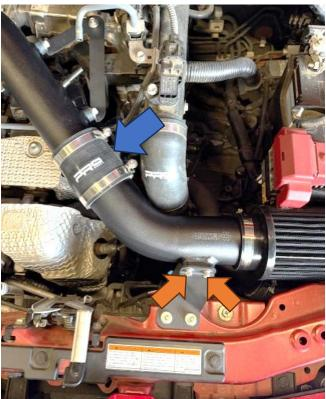
10. Now reconnect the vacuum line (blue arrow), secure the MAF sensor using the M4 bolts provided and once secure, reattach the MAF cable (orange arrow).
