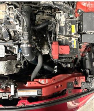
6. Locate the two M6 threads on the slam panel that were originally used for the OEM air feed. Screw the supplied anti-vibration rubber fixings in place and then secure the AIRTEC Motorsport mounting bracket with the two M6x10mm bolts and washers provided.
