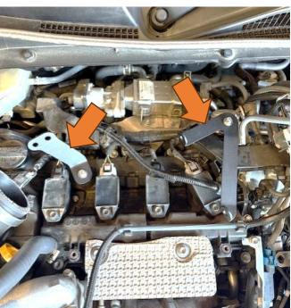
8. Now you can fit the large induction pipe to the brackets by securing it in place using the four M6x12mm bolts with washers provided.
