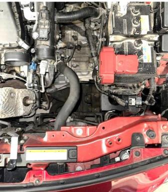
2. Undo the two 10mm bolts above the turbo headshield and disconnect the vacuum line (blue arrows)
