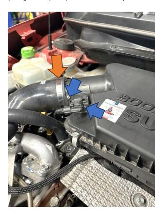
4. Disconnect the two wiring connectors and then carefully unclip them from the metal mounting bracket. You can then reattach them to the underside of the bracket in the same holes and reconnect them, as shown.
