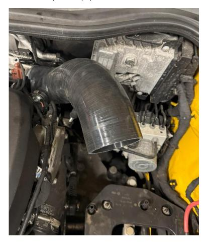
6. Finally, the AIRTEC Motorsport induction kit can then be fitted in place.
