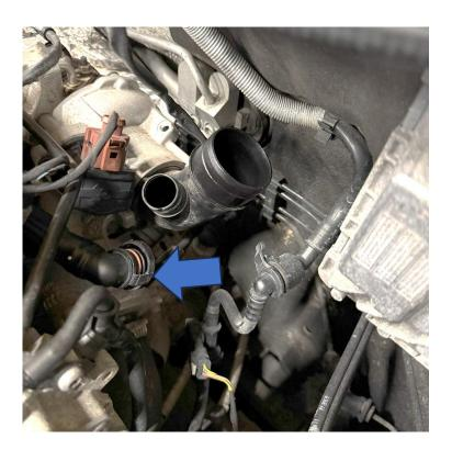
4. Apply a little grease to the O-rings on your new AIRTEC Motorsport turbo inlet adaptor before fitting it by rotating it anticlockwise to lock in place.
