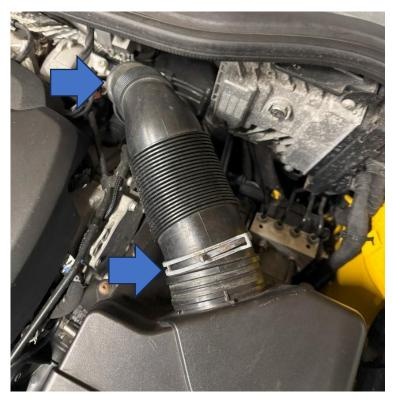
2. Locate and unhook the wiring loom clip connected to the original turbo elbow and undo the T27 Torx fitting attaching the elbow to the turbo.
