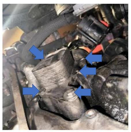
20. Install the AIRTEC Motorsport oil cooler adaptor reusing the original bolts.
