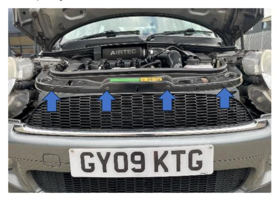
2. Now locate the outer clip on the bottom of the grille each side. Gently push these inward whilst pulling on the outer corner of the grille to release. Take care as they can become brittle and snap.
