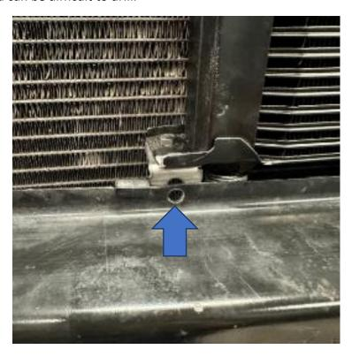
26. Now install both the lower brackets facing towards the front using two of the supplied M6x16mm bolts with Nyloc nuts and washers both sides, as shown. Then install onto the crash bar using the last two M6x16mm bolts with Nyloc nuts and washers.
