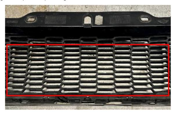
27. Reinstall the grille using the original outer push fit clips but replace the inner clips with the supplied M6 Button Head bolts with Mudguard washers and Nyloc nuts, as shown.
