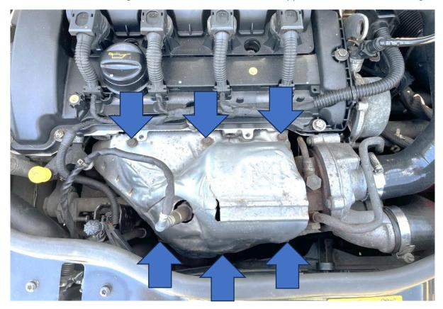
12. Undo the three 13mm nuts holding the downpipe to the turbo.
