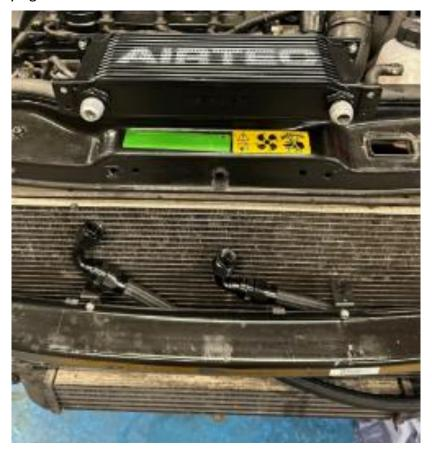
24. Temporarily locate the oil cooler in place using two of the original push fits from the upper grille (removed in Step 1) to hold it in place.
