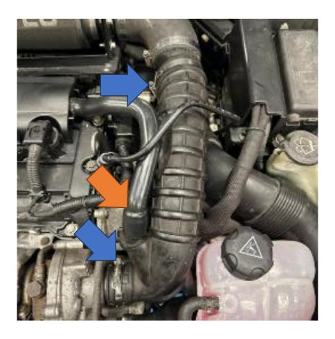
16. Loosen the two jubilee clamps securing the boost pipe and remove it from the car.
