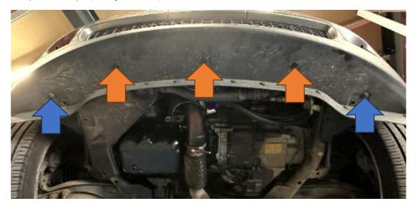
6. Each side, remove the three plastic push fit clips in the wheel arch (blue arrows) and pull the liner back to reveal a push fit clip (orange arrow) that holds the outer arch trim in place. Remove this to then gain access to the T25 Torx bolt holding the bumper underneath the headlight (green arrow).
