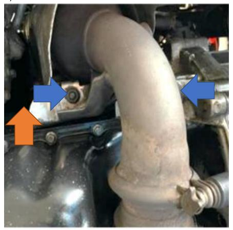
14. Working in the engine bay, remove the 8mm bolt holding the header tank in place and lift it to release it from the push fit below. Then move it aside and secure to allow access underneath.
