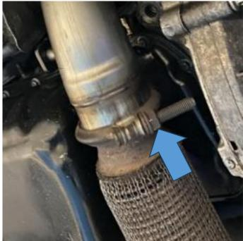
2. Undo the two 13mm nuts holding the downpipe brackets attached to the engine (blue arrows) and then remove. If there is not enough movement to free the downpipe, undo the 13mm nut attached to the bracket that was holding the left-hand downpipe bracket.
