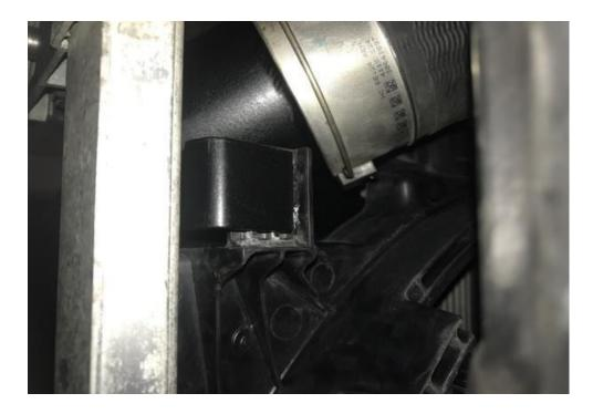
18. Bolt the intercooler to the radiator housing with the supplied M6 bolts with washers and then clip the boost pipes back to the intercooler.
