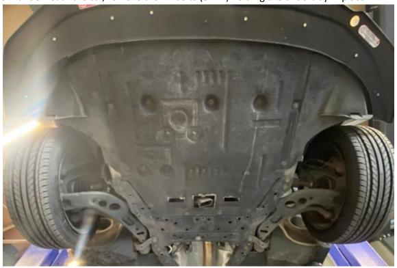
2. Each side, remove the two 8mm bolts from under the bumper and one 8mm bolt securing the inner arch to the bumper.
