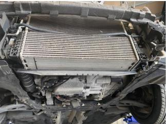
13. Undo the intercooler pipes by using a lever a flat-bladed screwdriver to release the clips. Then remove the T30 Torx bolts from each side of the standard intercooler securing it to the radiator. The intercooler can now be removed from the car.
