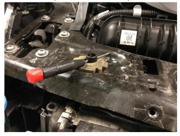
15. Remove the standard plastic air guides from the radiator pack by removing the T27 Torx bolts from the top of the air guide.
