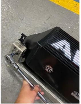
17. Lift the intercooler into place and loosely bolt the lower crossmember into place making sure the fan surround is located into the intercooler locating tabs.
