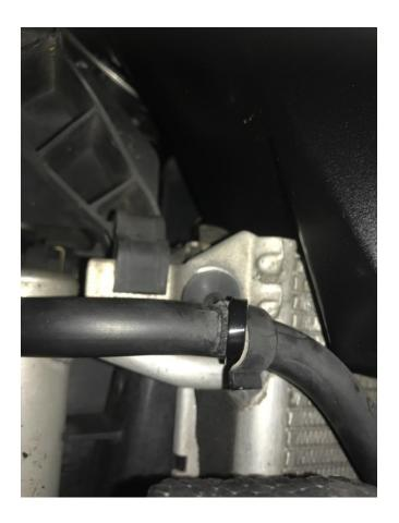
20. Finally, once happy with the fitment and clearance, fully tighten all bolts and refit the bumper in reverse of Steps 1 to 13.
