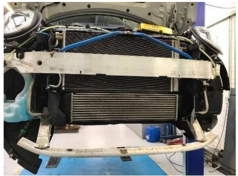
11. Unclip the bottom of the original intercooler by levering a flat-bladed screwdriver at the lower part of the clip.
