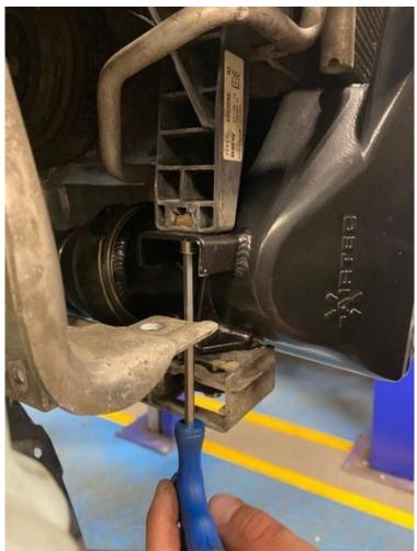
19. Cable tie plastic water pipe to securing clip – for added security to prevent rubbing.
