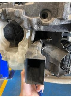
9. Remove the six 8mm bolts (three each side) from the sides of the crossmember and then remove the two T27 Torx bolts from the top of the crossmember.
