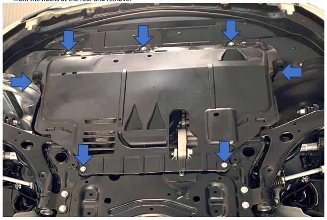
2. Locate the two holes highlighted on the subframe and use a 12.5mm drill bit to enlarge the holes.
