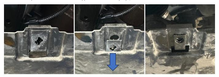
4. Finally, now fit the new under tray in place by reusing the four plastic holding clips. Secure the undertray in place using the eight supplied M6 button head bolts and washers.
