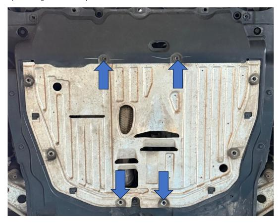
2. Next, undo the four rotation clips in each corner of the under tray. Then pull backwards to release it from the four plastic clips at the bottom and remove the undertray.
