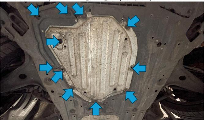
2. Fit the new AIRTEC Motorsport inspection panel in place using the eight supplied bolts and washers (blue arrows) together with the three original screw-type fixings that were fitted (orange arrows).
