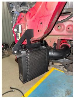
18. Attach the oil line with the 90-degree end to the rear fitting, as shown. Tighten it at the angle shown and then feed the line through the crash bar and down through the hole with the rubber trim fitted in Step 13.
