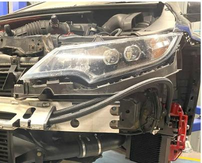
20. Now feed both lines past the left-hand brake duct, under the front panel and above the crossmember to reach the oil filter as shown. See Step 23 for where lines should locate once the under tray is removed.
