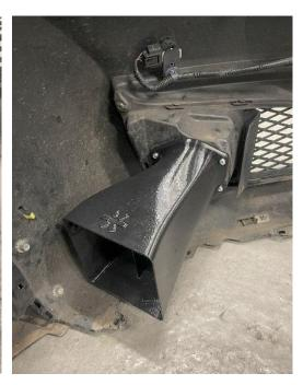
8. Add the scoop bracket as shown using the supplied M5x16mm Button Head bolts with nuts and washers both sides. The other end of the bracket mounts to the existing 10mm bolt on the inside of the bumper.
