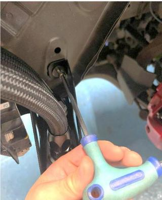
22. Working under the car, undo the service panel and then remove the off-side chassis brace for better access.
