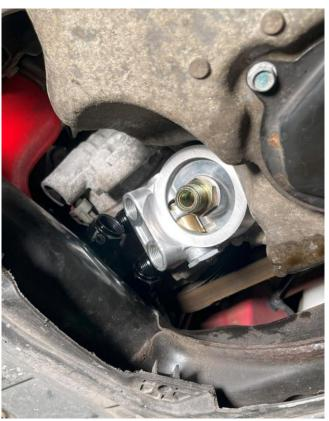
24. Once you have checked all the lines and fittings clear and do not touch the subframe, fully tighten them as well as the sandwich plate centre bolt. You can then add the supplied blanking fittings and then the oil filter. **Please note:** Make sure every fitting here is tightened all the way until it is firm and very tight.
