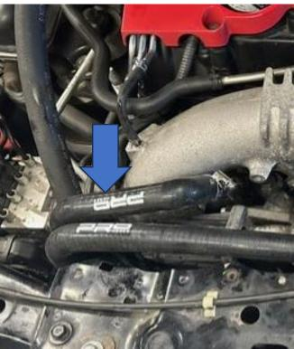
16. Use the supplied P-Clips with M6x16mm Button Head bolts and small Pan Washers to secure the first hose to the slam panel, as shown. Use the cable ties provided to secure the hoses together.
