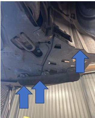
8. Locate the wheel arch fixings there are three screws at the bottom of the arch. Remove the clips holding the arch to the wing, these can break easily. Work around the shape of the arch and remove the last push fits. Once loose, untuck from the wing and remove the arch.
