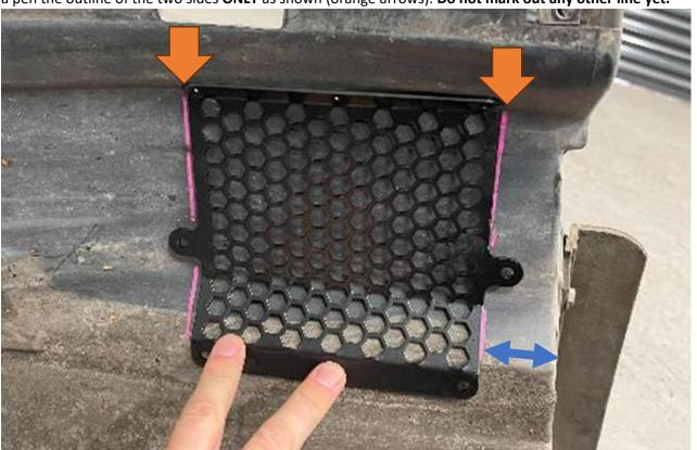
21. Now remove the mesh and mark out the cut lines, which will be 5mm further **inwards** than the two out lines previously made, as shown.
