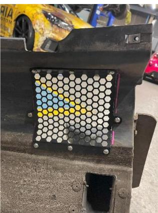
23. Check coolant level and the bleed system. You can then refit all parts removed. When fitting the bumper back, make sure to feed the new additional raidator scoop around the original brake duct.
