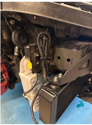
18. Remove the fog light and undo the plastic connector. Fit the supplied mounting bracket using the self-tapper provided and clip the connector onto the bracket.
