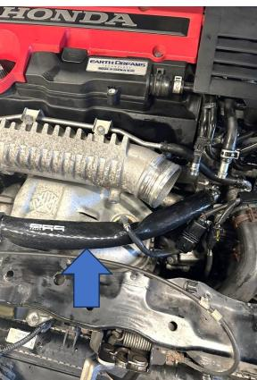
14. Run the hose along the slam panel and feed it down to the AIRTEC Motorsport radiator, as shown.
