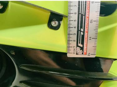
2. Measure 115mm from below the headlight to mark the top of the canard location.
