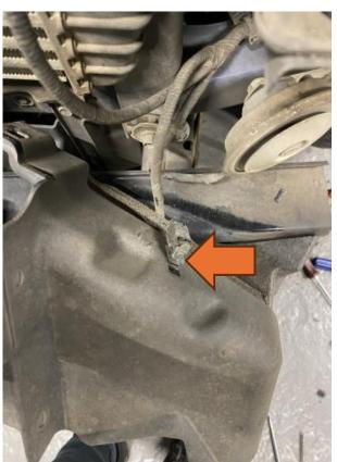
8. Remove the MAP sensor from the intercooler by undoing the T25 Torx bolt holding the sensor in.
