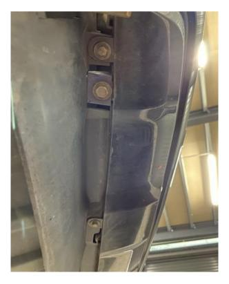
4. Now remove the four Philips screws securing the edge of the bumper to the inner arch liner each side.
