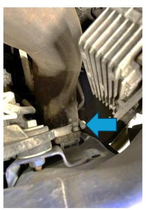
10. Now remove the intercooler by undoing the 10mm bolt and two 10mm nut securing each side in place.
