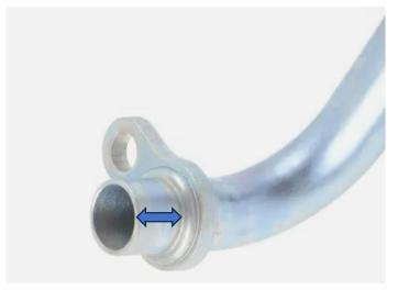
If this distance is more than 13mm it will need to be cut down OR the lines replaced.
