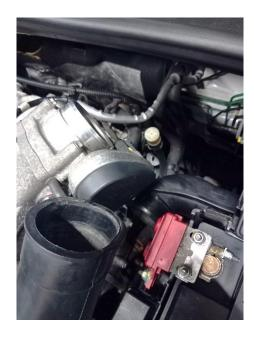
4. Loosen both battery terminals using a 10mm spanner and carefully lift the connectors off the terminals.
