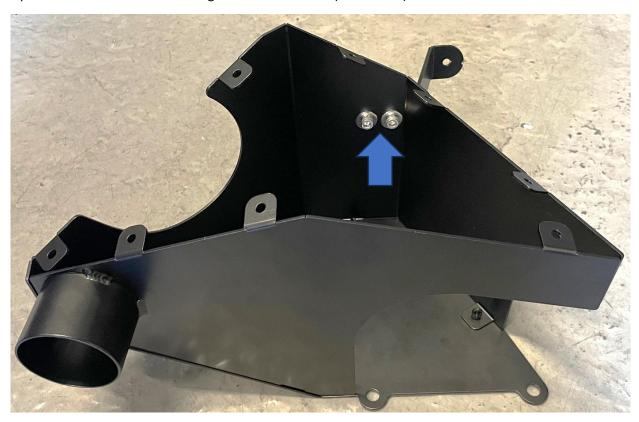
12. Attach the supplied aluminium locating pin onto the mounting bracket using the remaining bolt and washer, as shown.
