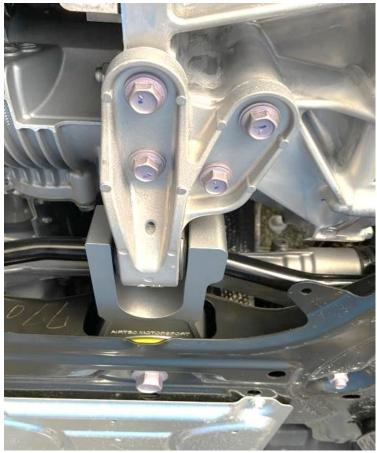
6. Finally, insert the new bolt provided into the torque mount and tighten, then reinstall the undertray.
