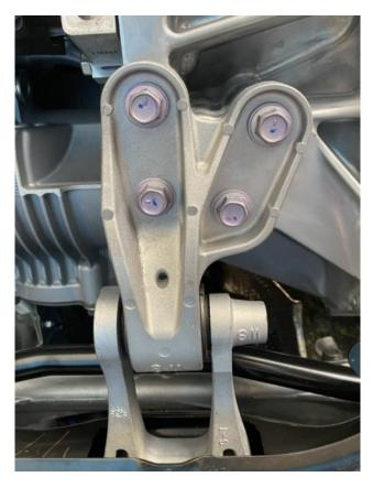
4. Install the new torque mount ensuring the insert is seated correctly as shown. Then reinstall reusing the original bolt.
