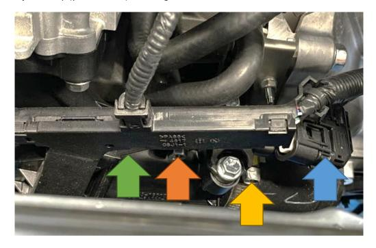
16. Undo the two 12mm nuts and two 12mm bolts (blue arrows) to loosen the inlet manifold. The throttle body has coolant lines going to it and so the inlet manifold cannot be remove from the car. Instead, rotate it to the right and position it so that you can get access to the throttle body elbow bolts. It is highly recommended you cover the inlet ports whilst you follow the next few steps to avoid the possibility of something dropping into it.
