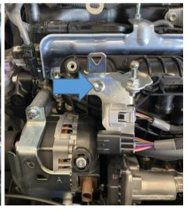
12. Locate the covered cable below the hoses as shown. Follow it along to the plug underneath and unclip it by pushing the blue button and pulling the plug backwards.
