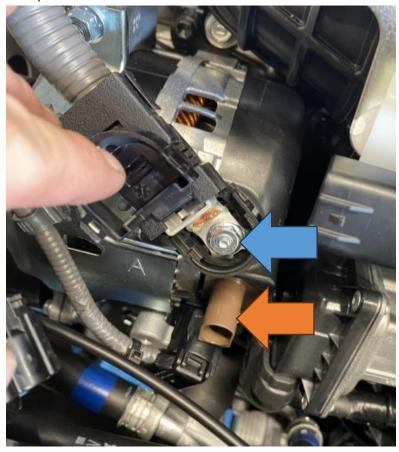
8. Undo the 10mm nut (blue arrow) and then release the push clip (orange arrow) holding the wiring harness in place. Fold the wiring loom back so it is out of the way.
