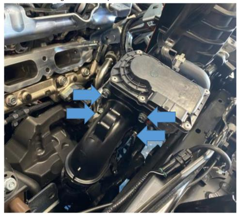
18. Undo the two 10mm bolts holding the MAP sensor to the elbow and swap it on to your new AIRTEC Motorsport elbow re-using the original bolts. Remove the gasket (orange arrow) from your original and place it into the groove on your new one.
