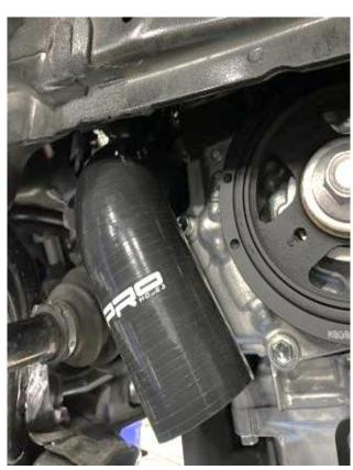
24. Finally, install the new pipe and once happy with the position reuse the original bolts to install on to the car, tightening the left-hand bolt first. Once installed and happy with the positioning tighten the jubilee clips. You can then refit the wheel arch panel and then refit I the undertray in reverse of removal.
