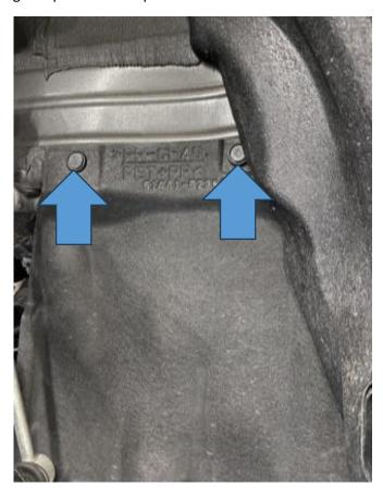
22. Locate and undo the jubilee clips securing both the silicone hoses to the intercooler and to the turbo. Then undo the two 10mm bolts securing the pipework to the car and remove the whole assembly.
