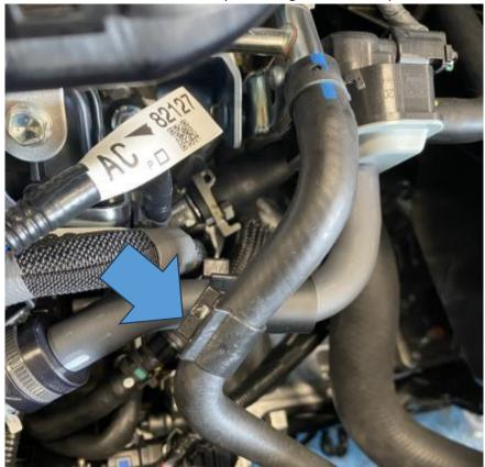
10. Undo the three 10mm bolts holding the coolant hard pipe above the inlet manifold and move the pipe back so that it is out the way.
