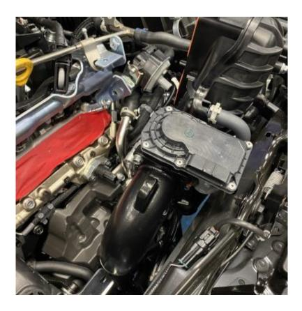
20. Connect the supplied silicone coupler with the jubilee clips provided onto the end of the throttle body elbow and then install the larger/straighter aluminium hard pipe supplied in the kit using the M8 Cap head bolt and washer provided. You can then connect the larger supplied silicone hose to the intercooler with the jubilee clips provided and once happy with the positioning fully tighten.
