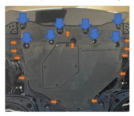
2. Now remove the four 10mm bolts holding the exhaust shield on.
