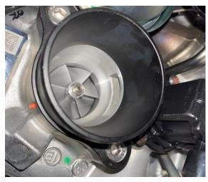
6. Once the flange is secured in place, you can install the supplied Pro Hoses silicone pipe with the longer end going to the intake and the shorter end to the turbo. Install using the jubilee clips provided.
