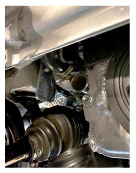
4. To remove the elbow, access it from both the arch liner as well as the rear of the engine where the exhaust shield was located. Start by removing the 10mm bolt on the flange (blue arrow), then remove the 10mm nut below and then remove the stud using an E8 socket (orange arrow).
