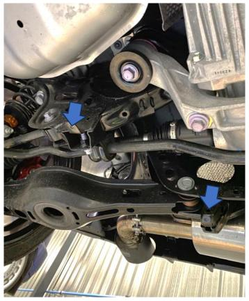
2. Now install the cooling guide by securing the front in place using the provided M6x20mm Socket Head bolt with a washer. Do not fully tighten yet as you will need some movement to align the rear.
