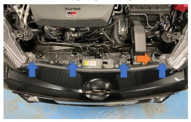
4. Inside each arch liner, remove the plastic push fit trim clip and then carefully unclip the two trim clip tabs and pull them apart to release each side of the bumper.
