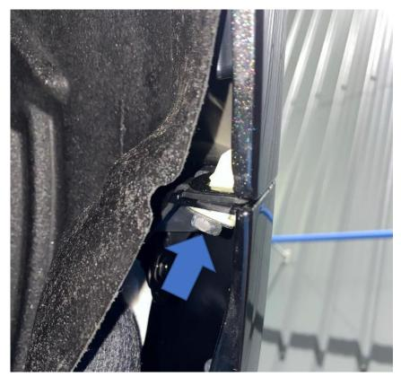
6. Carefully but firmly pull the edges of the bumper to release. Then, with the help of a second person holding the bumper, disconnect the plugs each side for the fog lights. The bumper can now be stored safely. Remove the foam support from the crash bar, this simply pulls off.
