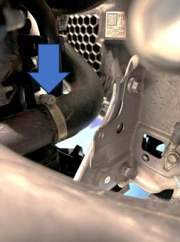
13. Remove the three 10mm bolts holding the intercooler to the car. You will then be able to remove the original intercooler along with the hot side/left-hand hose.
