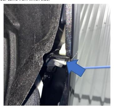
6. Pull the edges of the bumper to release and whilst a second person holds the bumper disconnect the plugs for the fog lights each side. The bumper can now be stored safely.
