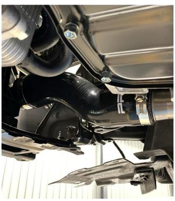
18. Reinstall the air guides removed in Step 9 reusing the three plastic clips and then install the air temperature sensor in the hole that was previously used for the wiring clip.
