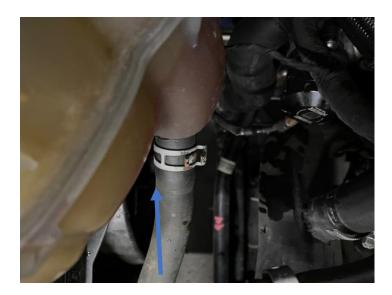
4. Install your AIRTEC Motorsport header tank in reverse of removal and use the original cap from the old header tank. You will need to add the supplied overflow to the header tank; to do so simply screw the threaded piece into the back of the tank just below the back of the coolant cap and then slide the overflow pipe onto it and point it down towards the underneath of the car.
