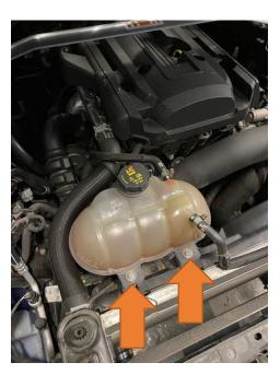
2. Remove the coolant lines to top of the bottle. Make sure that when these are removed you have something to hand to catch any spillage and something to plug the coolant lines with so they can be set aside without leaking excessively.
