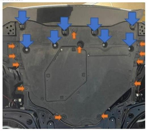
Still working under the car remove the five 10mm bolts on either side holding the arch liner to the front bumper.
