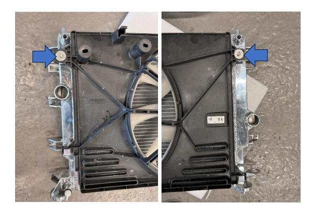
15. Again, with the help of a second person install the cradle onto the radiator and then lift it all into the car. As it is lifted into place ensure the top rubbers sit in their correct holes and then tighten the four 10mm bolts.
