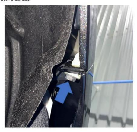
6. Carefully but firmly pull the edges of the bumper to release. Then, with the help of a second person holding the bumper, disconnect the plugs each side for the fog lights. The bumper can now be stored safely.
