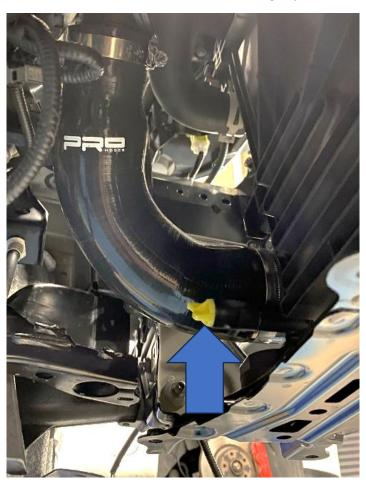
8. You need to remove the air box or induction kit to gain access to the upper radiator hose. Please see our <u>induction kit fitting instructions for help</u>. You can then remove the hose by releasing the clamp. Then locate the two smaller hoses going to the top of the radiator on each side and undo the clips to remove.
